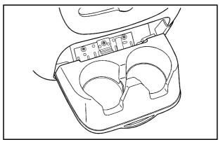
Pull downward on the lid to access the rear floor console cupholders.
